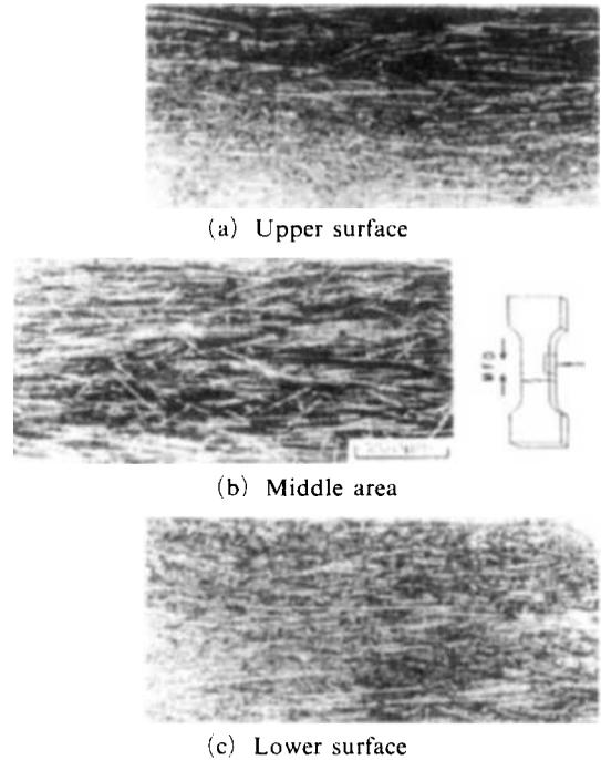
**Fig. 3** Photomicrographs taken on fiber orientation in the parallel plane of injection molded PPS parent.
