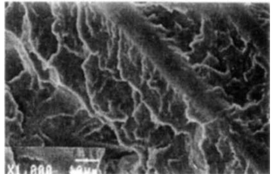
Fig. 13 Fatigue crack initiation and propagation of PPS weld at interface of fiber and matrix
